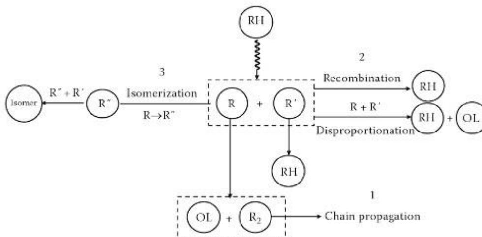
In the presence of bentonite crude oil under gamma – radiation changes the structure and obtained branched-chain paraffin (RH) via olefins (OL).
