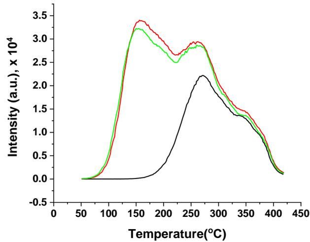
Fig. 1 TL intensity of irradiated natural feldspar with a dose rate of (2) 3.45 mGy/s; and (3) 92.07 mGy/s. The total dose for both samples was 33 Gy. Curve (1) represents the TL spectrum of natural feldspar not irradiated under laboratory conditions. The heating rate of TL measurements is 20°C/sec.
