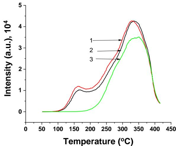
Fig. 2 TL intensity of irradiated natural quartz with a dose rate of (2) 3.45 mGy/s; and (3) 92.07 mGy/s. The total dose for both samples was 33 Gy. Curve (1) represents the TL spectrum of natural quartz unirradiated under laboratory conditions. The heating rate of TL measurements 20 °C /sec
