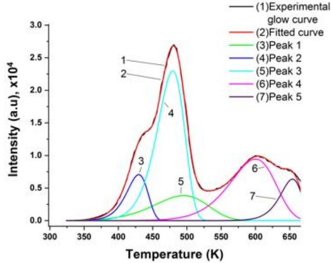
Fig. 3 Deconvolution of the TL glow curve of quartz irradiated at 20 Gy using GlowFit into five components. Natural quartz was heated at 650°C for two hours prior to irradiation.
