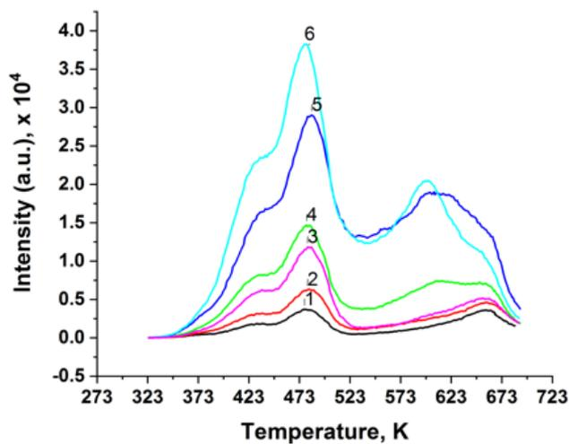
Fig. 2. Dose dependence of TL intensity irradiated quartz at different doses: (1) 2.24 Gy; (2) 4.48 Gy; (3) 7.72 Gy; (4) 11.40 Gy; (5) 17.92 Gy; (6) 22.40 Gy. Natural quartz was heated at  $650^\circ\text{C}$  for two hours prior to irradiation.
