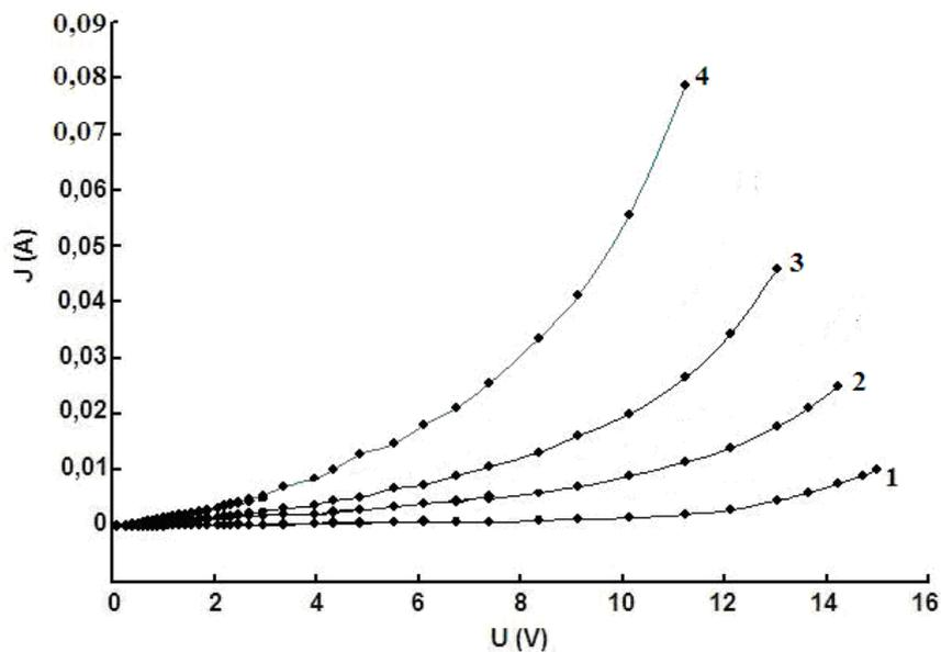
Fig. 2. VAC of the  $TlGaTe_2$  crystal perpendicular to the tetragonal axis "c" at temperatures; 1- 90K, 2- 120K, 3- 200K and 4- 300K.
