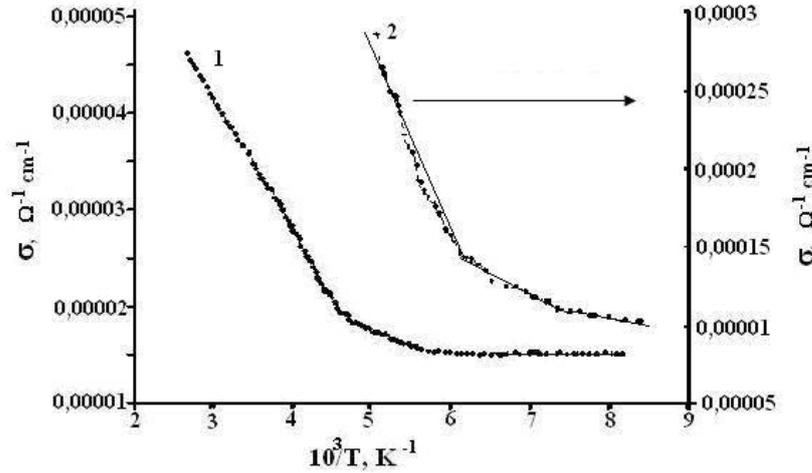
Fig. 3. Temperature dependence of electrical conductivity for a TlGaTe<sub>2</sub> single crystal (1-initial, 2-250 Mrad)
