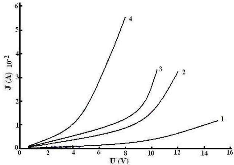
Fig. 1. VAC of the  $TlGaTe_2$  crystal along the tetragonal axis "c" at temperatures; 1- 90K, 2- 120K, 3- 200K and 4- 300K.
