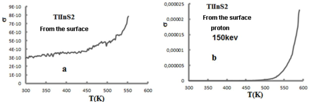
Fig. 3. Temperature dependence of electrical conductivity  $\sigma(T)$  for TlInS<sub>2</sub> crystals (measurements were performed along the tetragonal axis “c”. a - without irradiation; b - exposed to proton influence - 150 keV)
