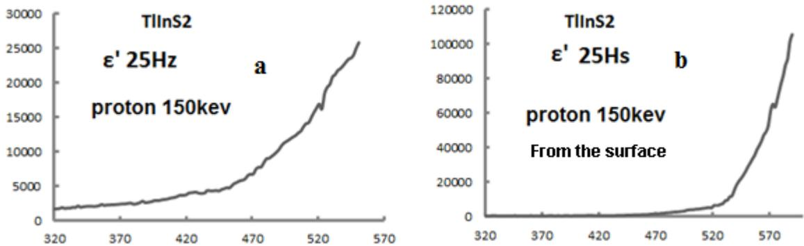
Fig. 2. Temperature dependence of permittivity  $\epsilon(T)$  for TlInS<sub>2</sub> crystals (a - perpendicular to the tetragonal axis “c” of the crystal; b - along the tetragonal axis of the crystal)
