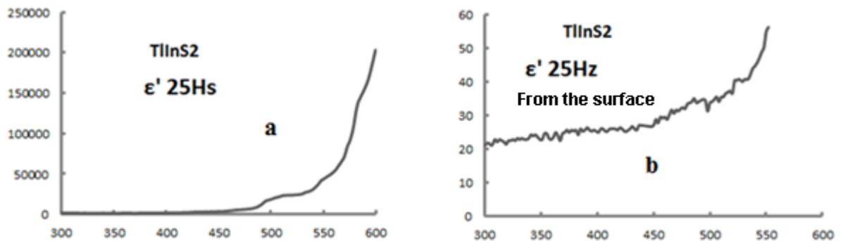
Fig. 1. Temperature dependence of permittivity  $\epsilon(T)$  for TlInS<sub>2</sub> crystals (a - measurements were performed perpendicular to the tetragonal axis “c”; b - measurements were performed along the tetragonal axis “c”).
