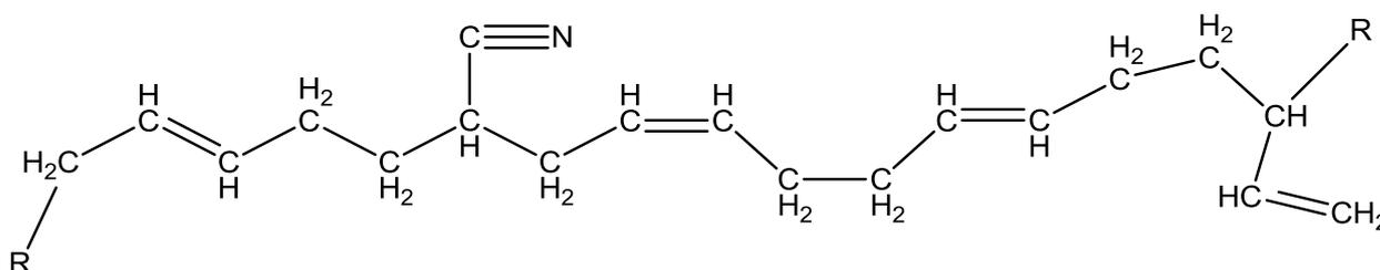
*Fig. 1. Scheme of nitrile butadiene rubber*
