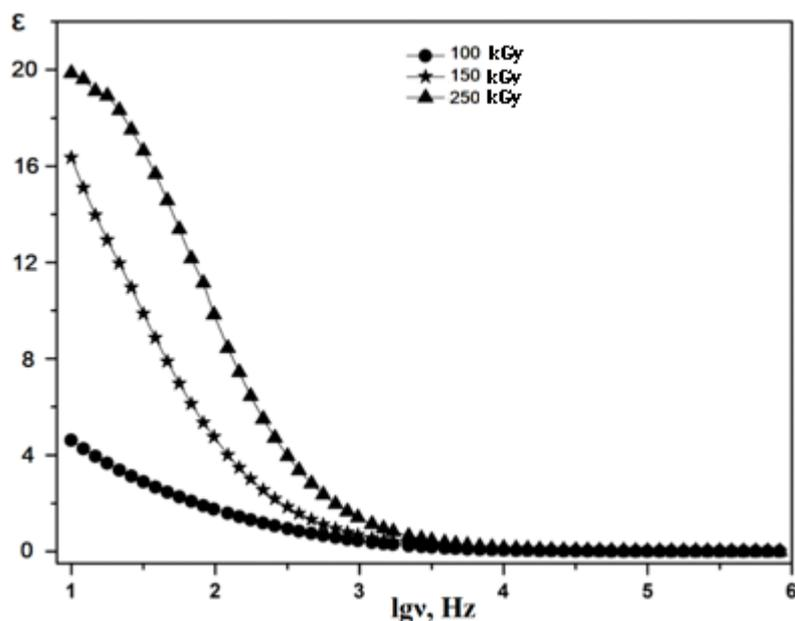
Fig. 2. Frequency dependence of the dielectric constant of irradiated nanocomposites (NBR + DSCB + ZrO<sub>2</sub>)
