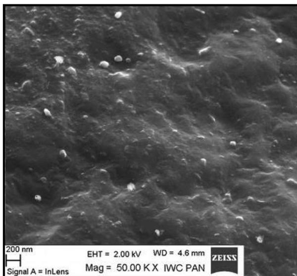
*Fig. 5. SEM image of the surface of the NBR / ZrO<sub>2</sub> / DSCB nanocomposite lowed by gamma irradiation by a dose of 250 kGy.*
