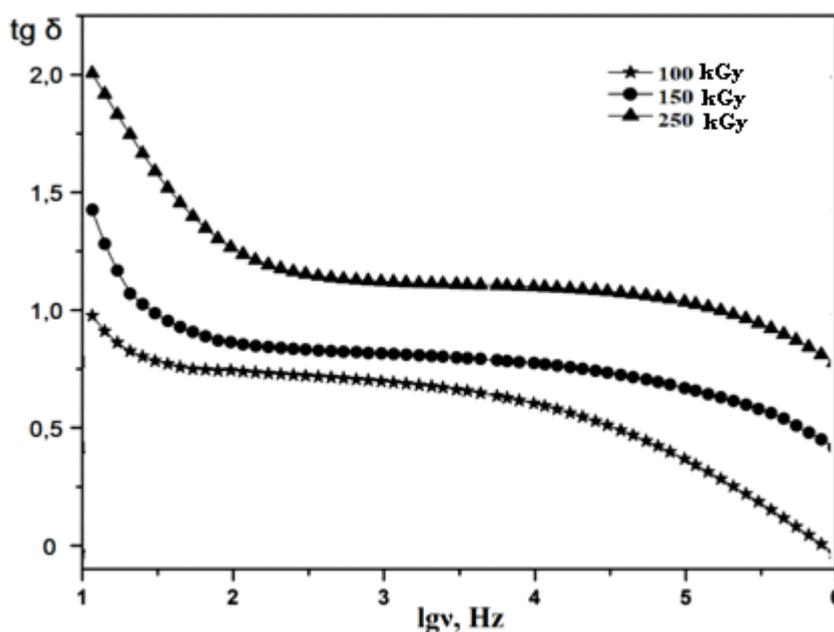
Fig. 3. Frequency dependence of the dielectric loss tangent of irradiated nanocomposites (NBR + DSCB + ZrO<sub>2</sub>)
