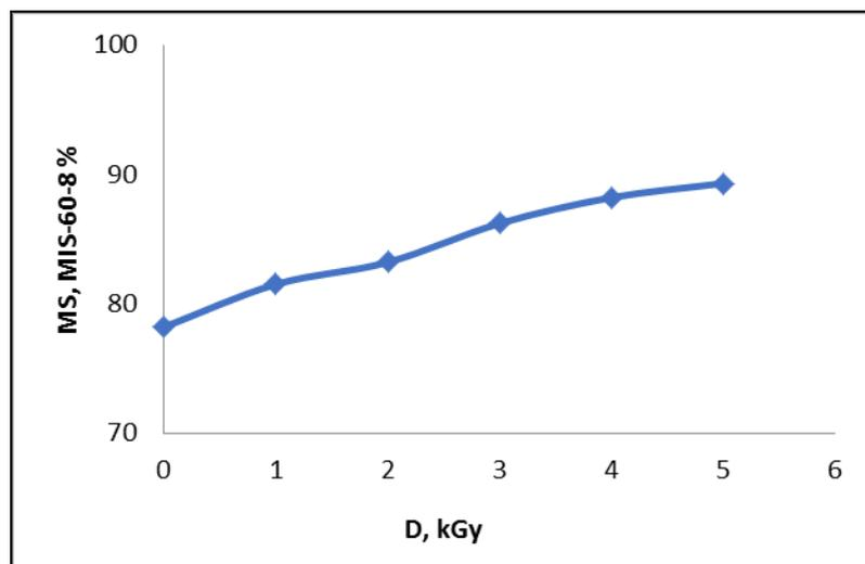
Fig. 4. Dependence of mechanical strength on absorbed radiation dose,  $T=450^{\circ}C$
