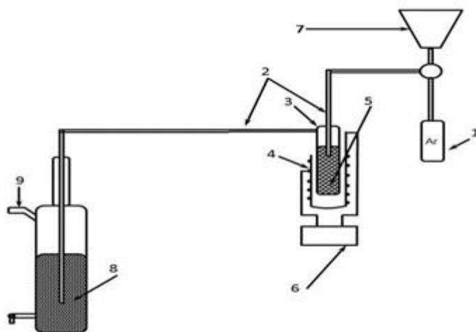
*Fig. 1. Scheme of an experimental device for producing activated carbon from semi-coke: 1 - gas cylinder; 2 - communication pipes; 3-reactor; 4 - spirals for heating the reactor; 5 - sample; 6 - temperature regulator; 7 - volume for water with a dispenser, 8 - gas meter; 9 - exit to the chromatograph.*
