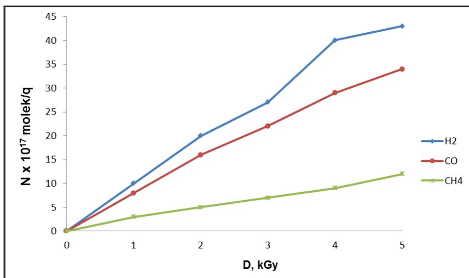
Fig. 3. Kinetics of H<sub>2</sub>, CO and CH<sub>4</sub> formation during radiation-thermal activation of coke in a water vapor medium, T=450°C
