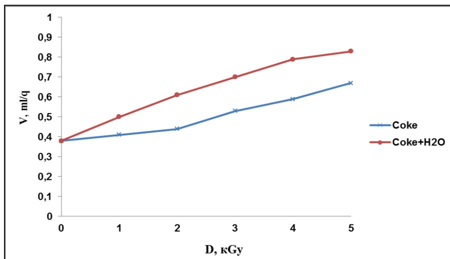
Fig. 2. Dependence of the sorption capacity of activated coke on the absorbed dose.
