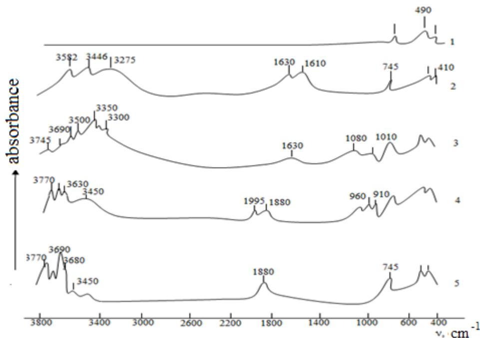
Fig. 1. Fourier IR spectra of nano-Zr treated at 673K (1), before and after exposure  $\gamma$ -radiation to the nano-Zr + H<sub>2</sub>O system at 300 (3), 473 (4) and 673 (5)
