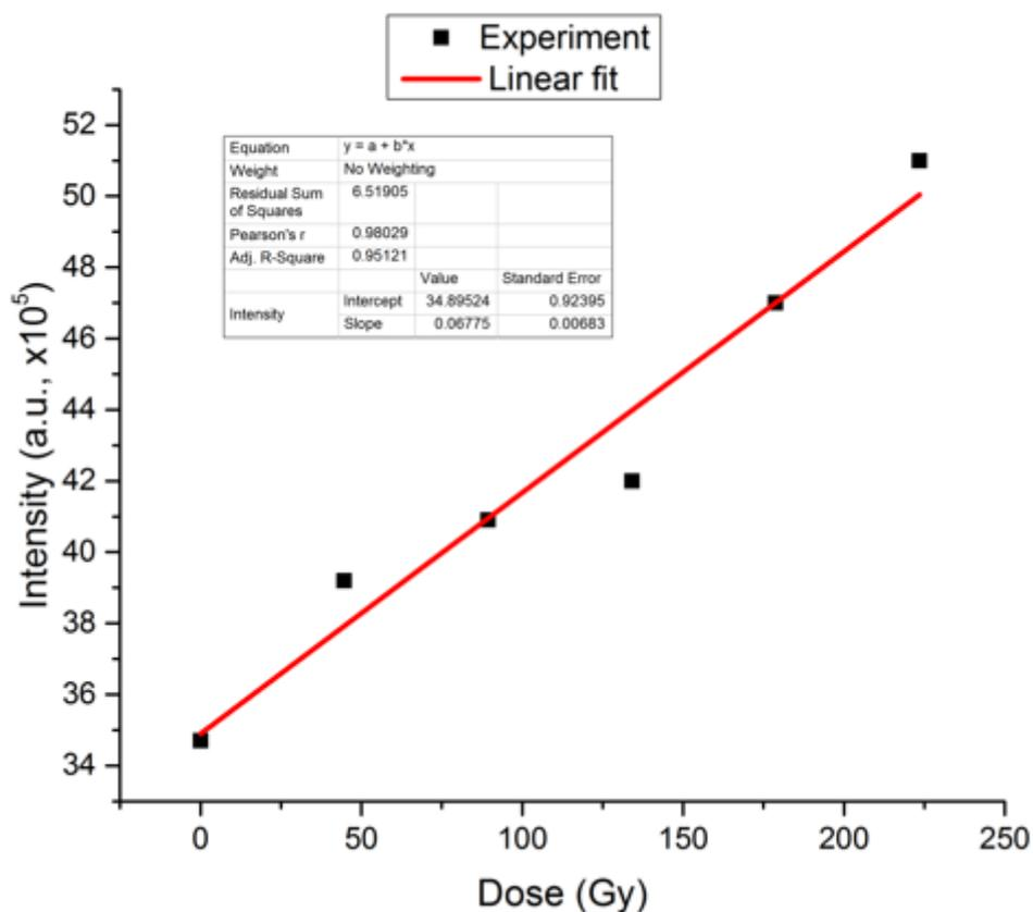
Fig. 2. Dose-response curve of fossil tooth enamel EPR spectra intensity. The intensity of EPR signal calculated conventional peak to peak height method. The curves were fitted with OriginPro 2018b.
