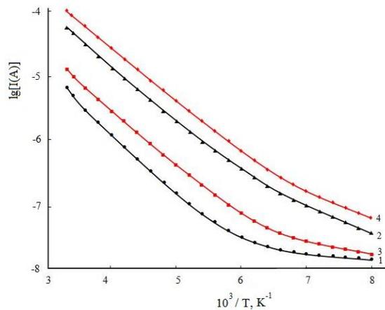
Fig. 3. Temperature dependence of current intensity ( $\lg I \sim \frac{10^3}{T}$ ) at different tensions in the dark for epitaxial film  $Pb_{1-x}Mn_xSe$  (p-type,  $x=0.01$ ) initial (1 and 2) and irradiated with  $\gamma$ -rays at 10kGy doses (3 and 4). 1,3-  $U=5$  V, 2,4-  $U=40$  V.
