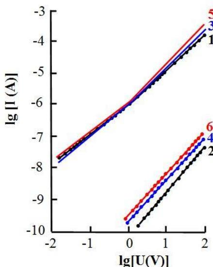
Fig. 2. VAC of epitaxial film of  $Pb_{1-x}Mn_xSe$  (*p*-type,  $x = 0.01$ ) initial (1 and 2) and irradiated with  $\gamma$ -rays in different doses, in the dark at different temperatures. 1,3,5 - 300K, 2,4,6- 125K. 3,4-10 kGy, 5,6 - 20 kGy.
