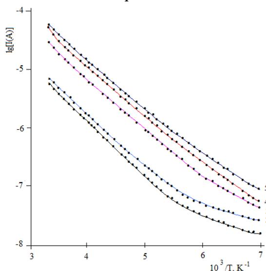
Figure 1. Dependence ( $lgI \sim \frac{10^3}{T}$ ) graph of current intensity on temperature at different intensities for epitaxial film of  $Pb_{1-x}Mn_xSe$  (p-type,  $x=0.01$ ). 1- 5V, 2- 10V, 3- 20V, 4- 30V, 5- 40V
