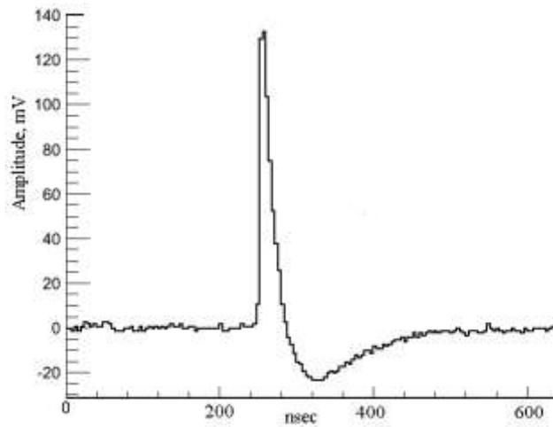
Figure 2: The recorded trace from the amplifier output.
