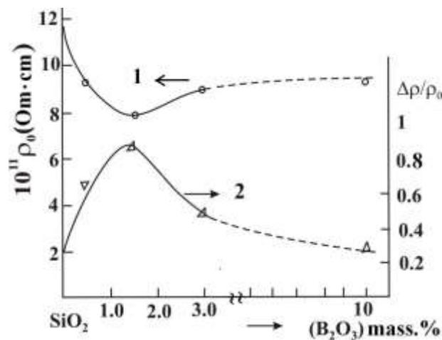
Fig.1 Dependence of resistance ( $\rho_0$ ) of unirradiated samples (1) and relative change of resistance ( $\Delta\rho/\rho_0$ ) of the  $\gamma$ -irradiated samples (2)  $B_2O_3/SiO_2$  at  $D=10\text{ kGy}$ .
