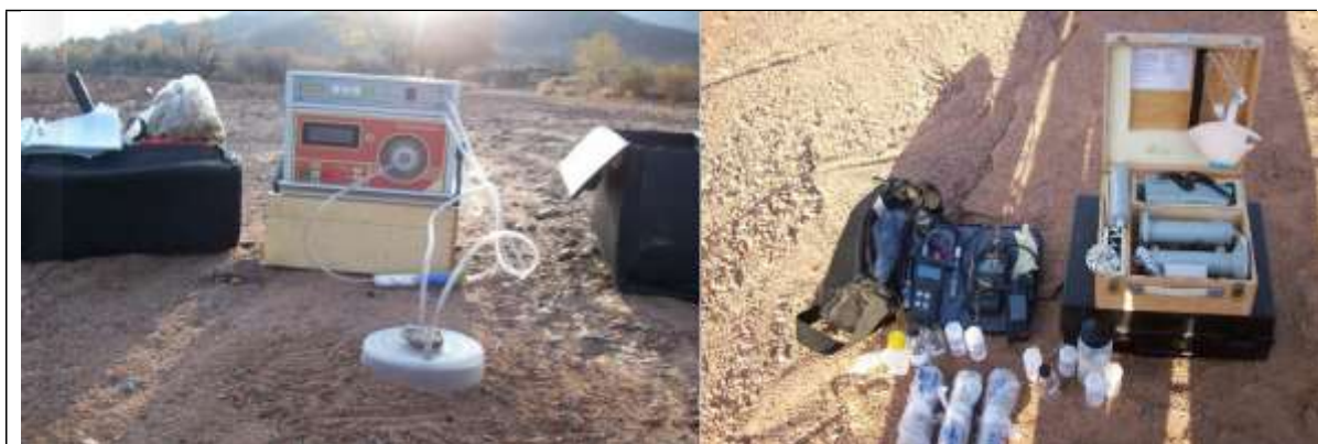
Fig. 3. The process of radon Rn^{222} measuring in soil cover
