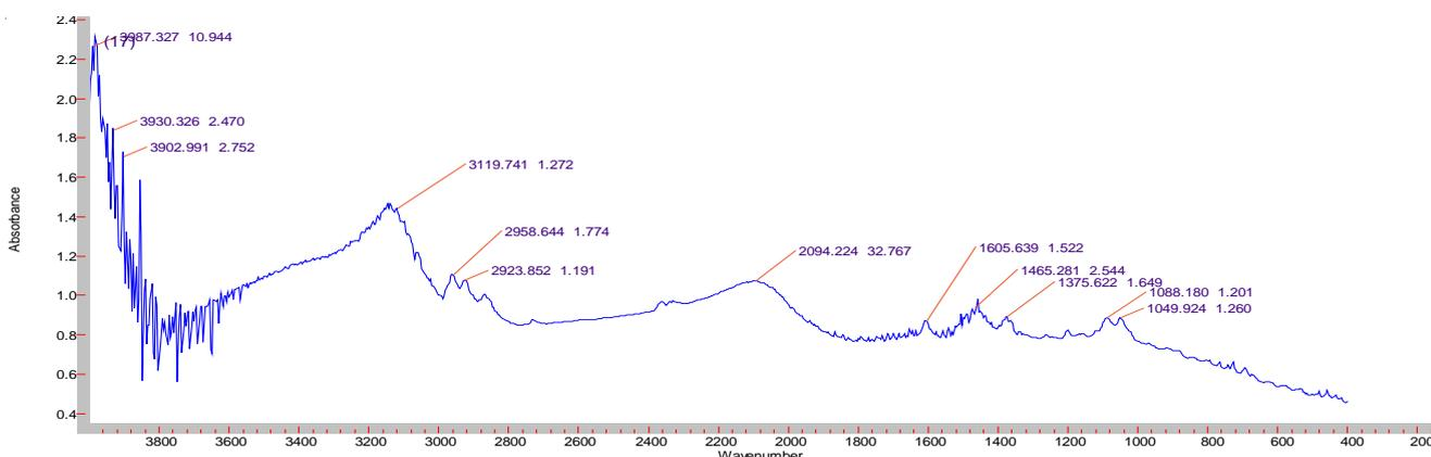
Fig.1 IR spectra of the original petrol
